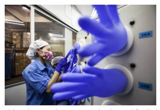
Employees attach latex gloves to an air compressor as other gloves are inflated in the air-leak test room at a Top Glove Corp. factory in Setia Alam, Selangor. PHOTO: BLOOMBERG
